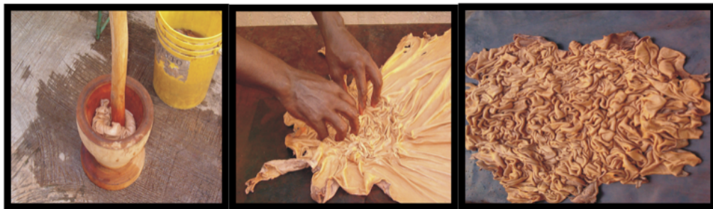
Plate 20: Pounding and Crumpling of leather
