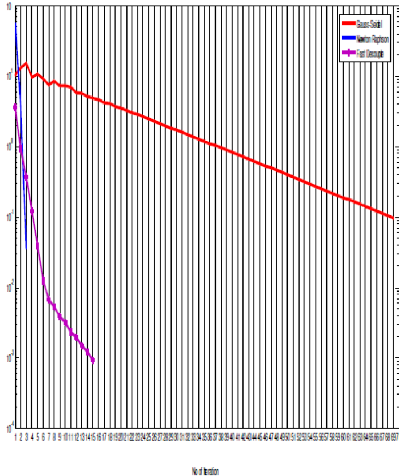
Fig.7: Absolute power mismatches as a function of the number of iterations for the 28-bus system
